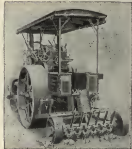
The Monarch Steam Road Roller with Steam Pressure Scarifier. A durable and dependable 3-wheeled 10-ton roller.
